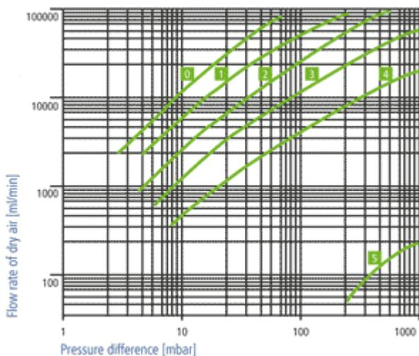
**Water flow rate related to pressure difference (filter plate dia. 30 mm)**
