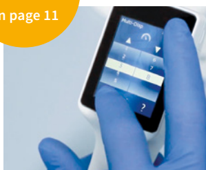
Setting the aspiration and dispensing speed
