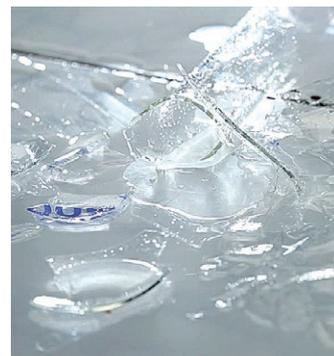
The PUR coating envelops the volumetric flasks like a protective skin.
