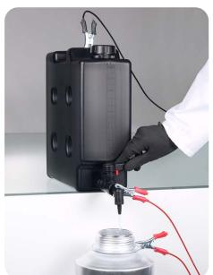
The compact jerrycan, made of electrically conductive HDPE, is especially well suited for use in explosion-proof areas. With a specific surface resistance of <105 ohms, the canister has a very high electrical conductivity. When correctly earthed, it prevents the danger of ignition due to an accumulation of electrostatic charge. The canister thus helps to meet the requirements of the ATEX 137, TRBS2153 and CENELEC 50404 guidelines.
