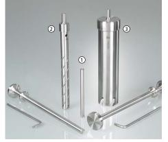
Meat sampler for microbiological sampling of carcass surfaces. The samplers for carcass sampling are similar to a cork drill. They can be used in the punch process (a destructive process, also called the cork drill or excision process) to remove a circular sample of tissue of 5 cm<sup>2</sup> from the surface. After the punch sample is cut out, it is removed from the carcass with a scalpel and tweezers.
