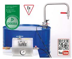
The withdrawal system can be used to dispense high-purity liquids quickly and without complications. An excess pressure is produced in the container with pressurised gas (compressed air or nitrogen), thereby pumping the liquid out of the tank. In this way, large amounts of hazardous media can also be safely dispensed and accurately metered. For use with media sensitive to oxygen or for ul-
