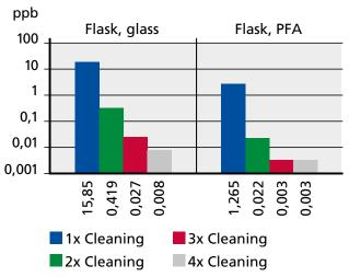
Cleaning of glass and PFA volumetric flasks after contamination. Source: Kali-Forschungsinstitut, K. Mangold
