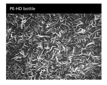
Pictures of the surface structure of PTFE, PFA, and PE-HD with a scanning electron microscope (8000 times magnification).
