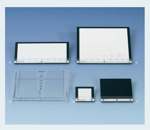
DESAGA Application Templates for all formats of plates  $a = for 200 \times 200 \text{ mm} \cdot b = for 200 \times 100 \text{ mm} \cdot c = for 100 \times 100 \text{ mm}$   $d = for 50 \times 50 \text{ mm} \cdot e = Application and Evaluation Template 200 x 200 mm$
