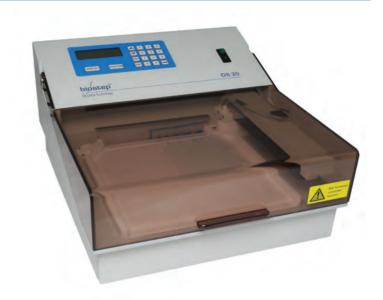
The spray methods define all important parameters, such as spray rate, volume to be sprayed and reagent selected. The free selection of X-Y coordinate direction means that it is possible to spray evenly, either individual tracks or areas of any size up to 200 x 200 mm.
