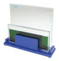
The dipping chamber is an alternative to spraying for avoiding environmental pollution. These chambers fulfil the established requirement: rapid and uniform implementation of a precise detection reaction. Special advantages of the dipping method are the improved uniformity of reagent distribution and the quick, reliable operation. The reagent is brought onto the plate - not into the air! All familiar spray reagents can also be used for dipping.
